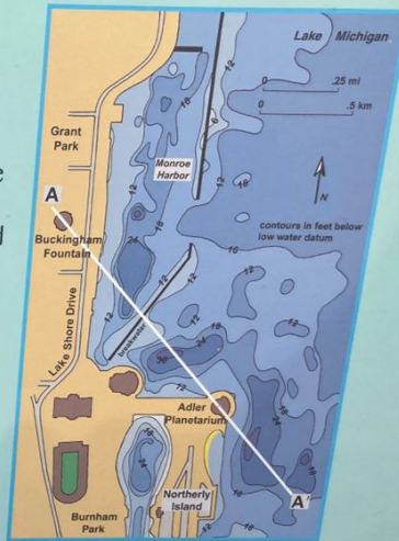
Cross section A-A' shows examples of lake-bottom depressions formed by dredging for clay fill in the vicinity of Monroe Harbor and Northerly Island.
